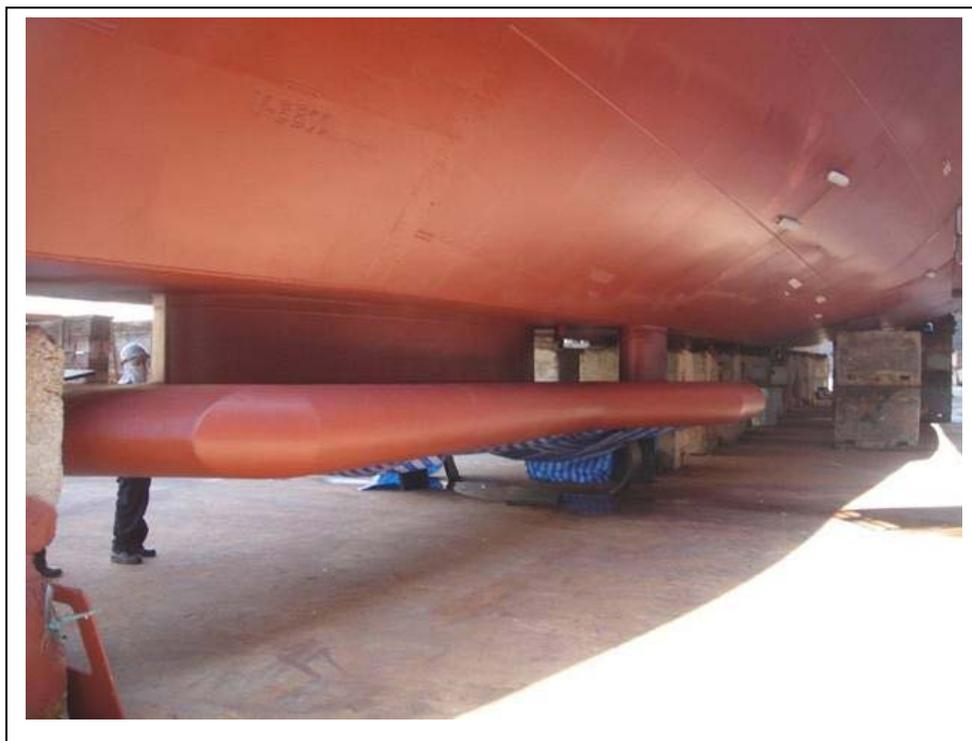
*Fugro collects multibeam echosounder data from specialist equipment housed in a gondola platform mounted beneath the hull of survey vessel Fugro Equator. Photo courtesy of Fugro.*
