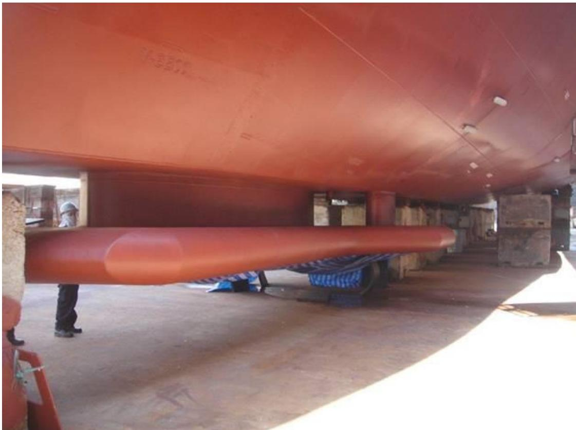
*Fugro collects multibeam echosounder data from specialist equipment housed in a gondola platform mounted beneath the hull of survey vessel Fugro Equator. Photo courtesy of Fugro.*
