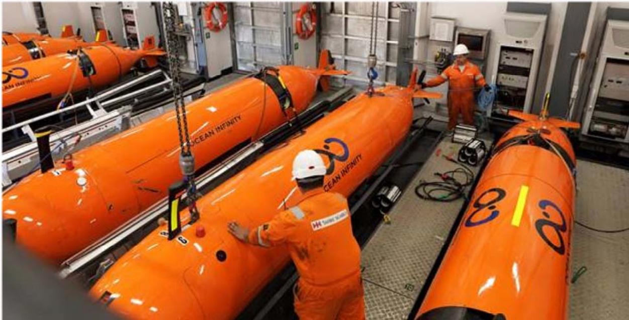
Ocean Infinity's AUVs being prepared to autonomously map the ocean floor, aboard Seabed Constructor
